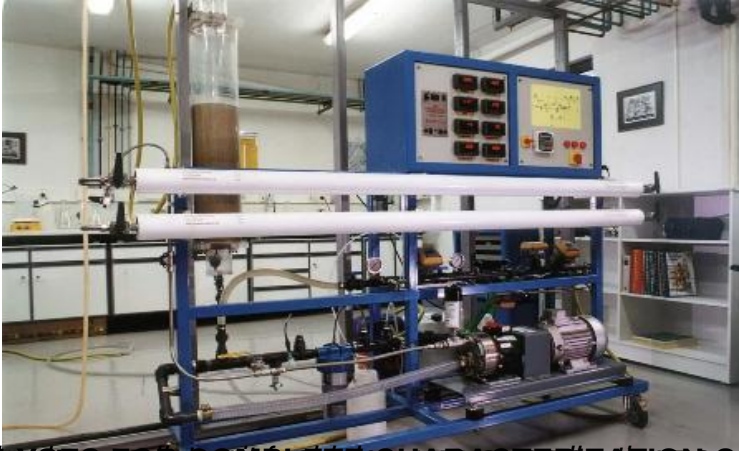
ADVANCED INSTRUMENTED TREATMENT OF WATER SOURCES with chemical addition for municipal and industrial wastewater, water softening and geothermal fluids from oil fields.
